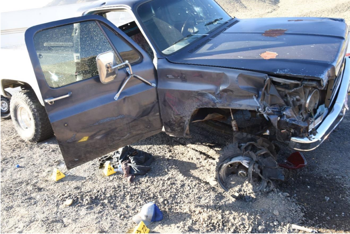
The damaged front passenger wheel of Williams' truck due to the spike strips as documented in Forensic Report #4.
